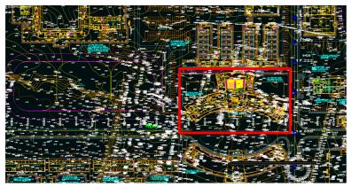
Step 2. Press "Trim" tab or type command "Tr", then enter. Click the rectangle and right click, then start erasing the drawings around it. If the drawings cannot be erased, check the layer tab and see if these layers are locked. Unlock it. If it is blocked, explode it.
